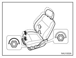
To adjust the height of the driver's seat cushion, turn the knobs located on the outboard side of the seat cushion.
